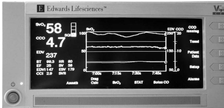
**Figure 4.2** • Continuous cardiac output and mixed venous oxygen saturation obtained from a Swan-Ganz catheter commonly used during off-pump surgery. (Image courtesy of Edwards Lifesciences, Inc.)
