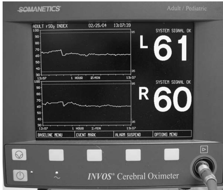
**Figure 4.1** • The Somanetics INVOS Cerebral Oximeter. This device uses near infrared spectroscopy to measure the regional oxygen saturation of predominantly venous blood directly in the brain through optical sensors placed on the right and left side of the forehead. (Image courtesy of Somanetics Corporation)
