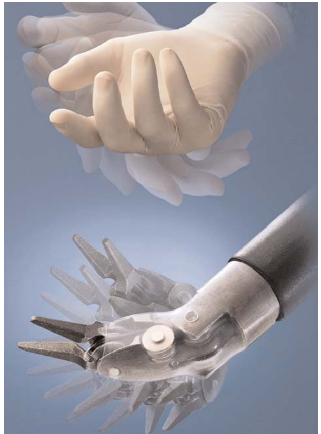
FIGURE 11-6. The da Vinci surgical EndoWrist provides articulation for surgical instruments.
