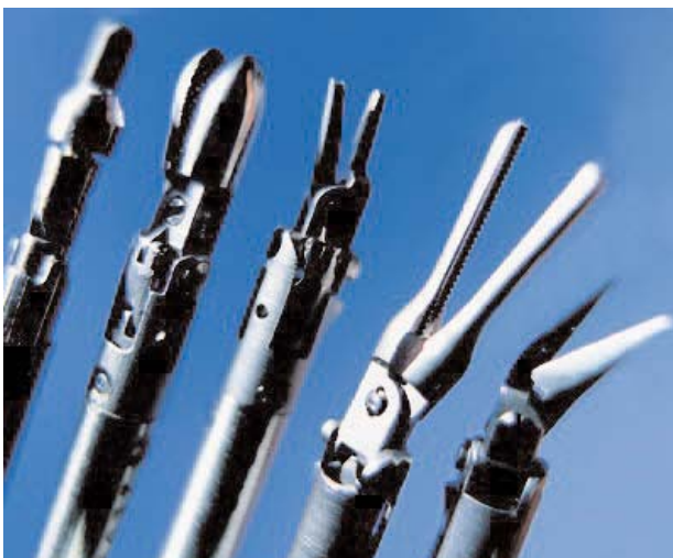
FIGURE 11-5. The ZEUS microsurgical instruments with jointed tips.
