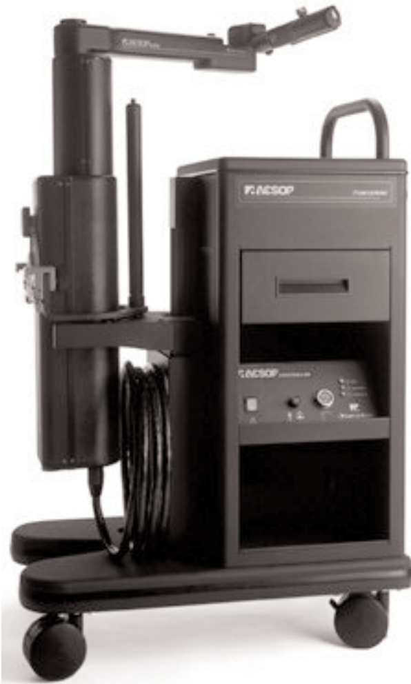
FIGURE 11-2. The AESOP robotic arm. It can be mounted to the operating table and accommodates most conventional endoscopes.
