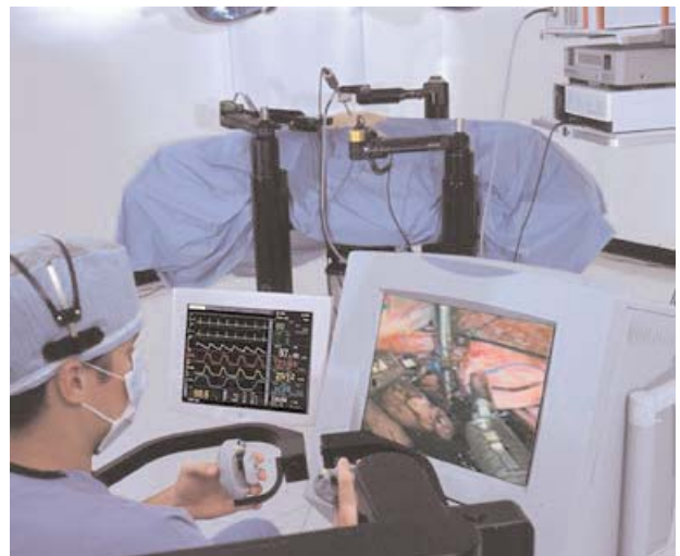
FIGURE 11-4. The ZEUS Robotic Microsurgical System. The three robotic arms are shown in the background, attached to the operating room table.
